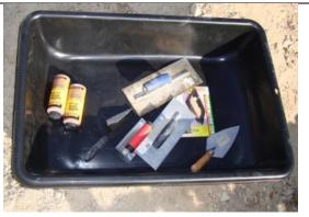
15. The other tools used were a plastic mixing tub, liquid cement color to make the concrete match the color of the stepping stones, and various trowels and spatulas to spread the concrete mix.
